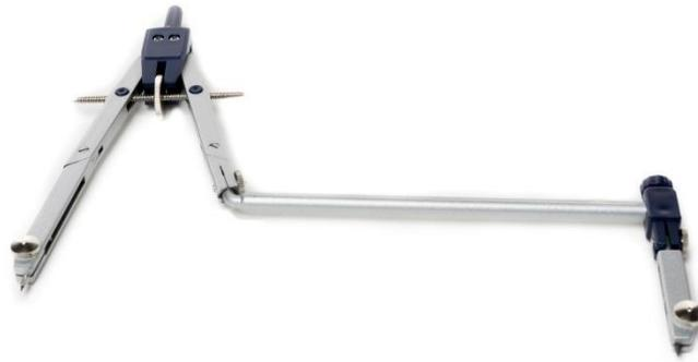
The biggest circle or arc you can make with the extension beam fully extended is 22 inches diameter<sup>2</sup>. The compass is not easy to control if you make the circle that large, but 20 inch diameter is easily managed. That's large enough to put a small goat through.
